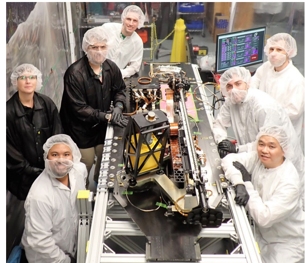
Fig. 1 The TRIDENT flight drill installed horizontally on the IM-2 Nova-C lander panel with a MSolo model temporarily installed for alignment.
